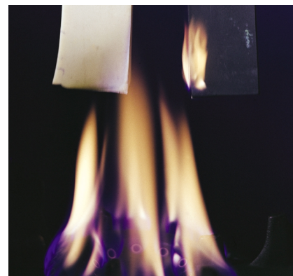
Flame resistance testing left: silicone rubber / right: organic rubber
